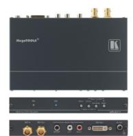
The **VP-471** is a high-performance digital scaler for 3G HD-SDI signals. It up or down-scales the incoming video to computer graphics, SD or HD video resolutions to a DVI connector and de-embeds the audio to S/PDIF and stereo audio on RCA connectors.
