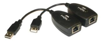
When used with a compatible transmitter, the Intelix AVO-USB-C extender transmits low and full speed USB signals over twisted pair cabling. The unit extends low speed USB 1.0 and 2.0 signals up to 330 feet, and full speed USB 1.0 and 2.0 signals up to 100 feet. Convenient connector dongles allow direct connection to the host and client devices, facilitating a clean, low-profile installation.
