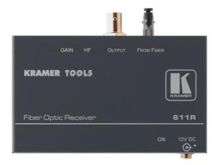
The 611T and 611R are a high-performance fiber optic transmitter and receiver for composite video signals. The 611T transmitter converts a composite video signal into a fiber optic signal and the 611R receiver converts the fiber optic signal back into a composite video signal.
