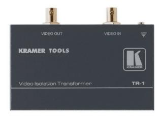
The TR-1 is a high-resolution video isolation transformer for composite video signals. It provides complete isolation between devices to eliminate video hum, ground loops, and DC offsets, which can degrade picture quality.
