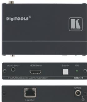
The **SID-H** is a twisted pair transmitter and step-in commander for HDMI and unbalanced stereo audio signals. The unit includes a "Step-In" button that allows the local source to be routed as the active source on the main display through the main switcher.
