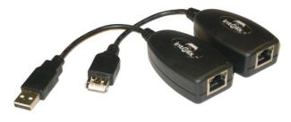
When used with a compatible transmitter, the Intelix AVO-USB-H extender transmits low and full speed USB signals over twisted pair cabling. The unit extends low speed USB 1.0 and 2.0 signals up to 330 feet, and full speed USB 1.0 and 2.0 signals up to 100 feet. Convenient connector dongles allow direct connection to the host and client devices, facilitating a clean, low-profile installation.
