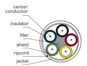
Kramer's BC-5X/LSHF is a high-resolution low-smoke, halogen free  $75\Omega$  5-mini coaxial cable perfect for routing RGBHV signals in commercial or residential A/V systems.
