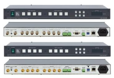
The VS-44HD and VS-44HDxl are high-performance 4x4 matrix switchers for HD-SDI and 3G HD-SDI signals, as well as a dual link 2x2 matrix switcher. Switching is implemented during the vertical interval period according to the SMPTE RP-168 standard, when using synchronized digital video sources.
