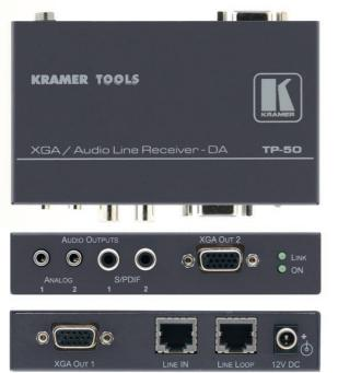
The TP-50 is a twisted pair receiver for computer graphics video and unbalanced stereo audio or S/PDIF audio signals. The unit converts the twisted pair signal back into two computer graphics video, stereo audio and S/PDIF audio signals simultaneously.
