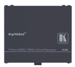
The 648 is a high-performance bidirectional optical repeater for FireWire® 1394a and 1394b signals. When used in pairs, it extends FireWire® cable runs up to a distance of 500m.
