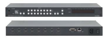
The **VS-88H** is a high-performance matrix switcher for HDMI signals. It reclocks and equalizes the signal and can route any input to any or all outputs simultaneously.
