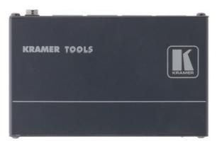
The VM-3AN is a high-performance distribution amplifier for balanced stereo audio signals. The unit takes one stereo input and distributes the signal to three identical outputs.
