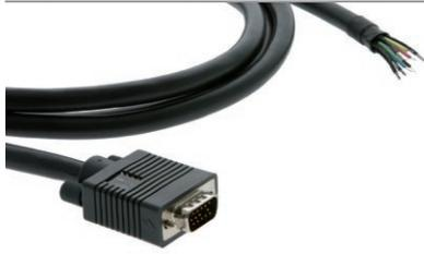
Kramer's computer graphics video installation cables are constructed of 5 mini coax cables in a single jacket with a 15-pin HD (M) connector at one end and 5 bare mini coax cables at the other. They are used for cable runs which require an easier pull through walls, conduit, furniture, etc.
