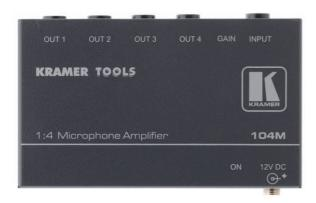
The 104M is a high-quality distribution amplifier for dynamic microphone signals. It takes a microphone input and distributes the signal to four identical line-level outputs.
