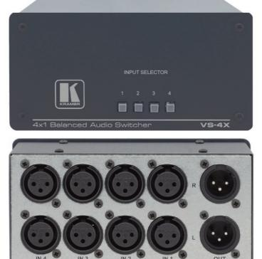
The VS-4X is a high-performance switcher for balanced stereo audio signals on XLR connectors. It switches any one of four stereo signals to a single stereo output.
