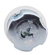
The SPK-CC688 are two-way speakers designed for mounting in the ceiling. They have a closed back design with a 8-inch metal can and aluminum grilles. The dualdriver coaxial speakers are designed with transformer and behind-the-grille power selector switch with either direct  $8\Omega$ or 70/100V room balancing.
