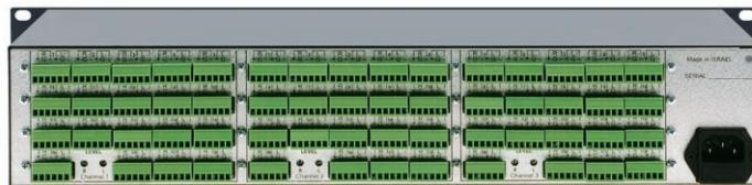
The **VM-54A** is a high-performance distribution amplifier for balanced stereo signals. It can also be configured as three 1:18 distribution amplifiers for balanced stereo audio.
