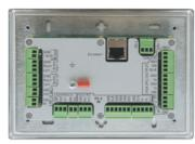
The WP-501 is a switcher for computer graphics video, composite video, stereo audio and microphone signals. With some of its input connectors placed on the back panel, it perfectly fits rooms with permanently installed PCs and video sources. It routes one of three AV input sources (one front & two rear) to a display and controls the display by IR or RS-232 commands.
