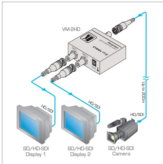
The **VM-2HD** and **VM-2HDxI** are high-performance distribution amplifiers for HD-SDI and 3G HD-SDI signals. The units take one input, provide reclocking and equalization and distribute the signal to two identical outputs.
