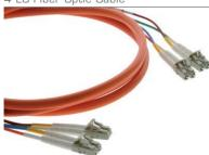
Kramer's 4LC fiber optic cables are constructed of 4 individual color coded multi-mode 50/125um simplex cables of 2.0mm diameter each, contained in a round overall orange jacket. They are intended primarily as companion to various Kramer detachable transmitter/receiver sets.
