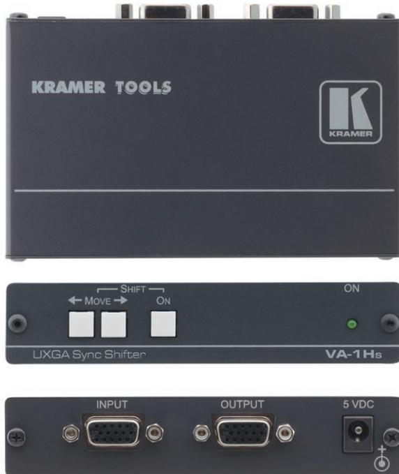
The **VA-1Hs** (previously VA-1H) is a high-performance line driver as well as picture shift corrector that can be used for any computer graphics video signal from VGA to WUXGA. The unit compensates for sync delay on long lines by shifting and rebuilding the sync so that the picture is properly displayed. The shift correction is saved in nonvolatile memory.
