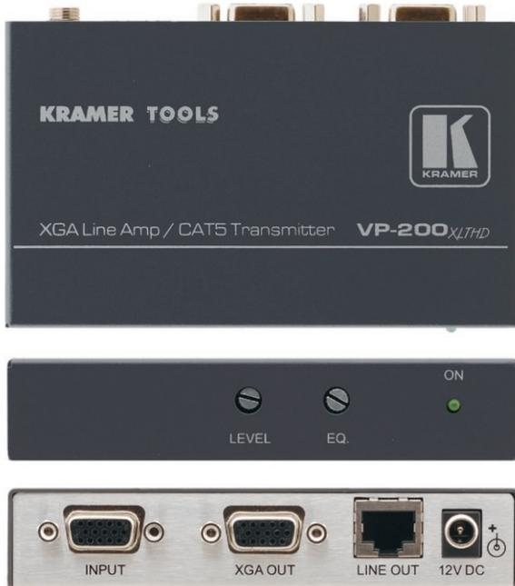
The **VP-200xITHD** is a high-performance line and distribution amplifier for computer graphics video signals with resolutions ranging from VGA through UXGA and HDTV. It takes one computer graphics video or HDTV input and provides one line-amplified output on a 15-pin HD connector and one twisted pair output on an RJ-45 connector.
