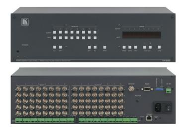
The **VP-885** is a high-performance universal matrix switcher for composite video, s-Video (Y/C), component video (Y, Pb, and Pr), balanced stereo audio and S/PDIF digital audio signals. It can route any or all inputs to any or all outputs simultaneously.
