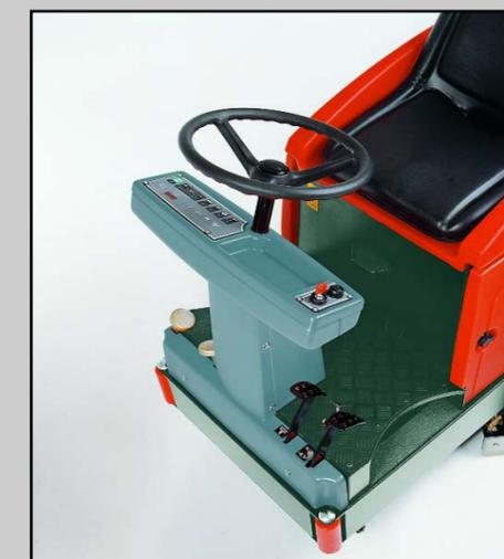
**Operator compartment:** The operator can access the driver's seat from both sides with an excellent view of the area to be cleaned. All operating elements are in direct view and easy reach of the operator. Adjustable, comfortable driver's seat.
