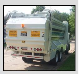
The Kann Up and Over Recycler is equipped with a standard 2 yd<sup>3</sup> bubble tailgate for added capacity.
