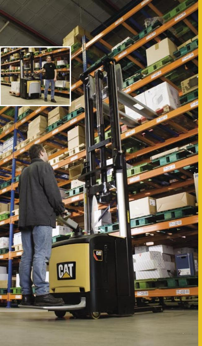
(Pictured from left to right) The poweRamic mast affords excellent overall visibility for safe operation and precise load handling.
