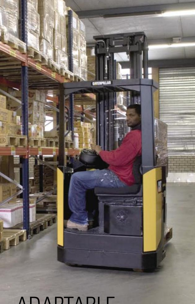
(Pictured far left, from top) The **NSV12-16NI** range of platform stackers include Initial lift (I) versions for handling two pallets simultaneously.
