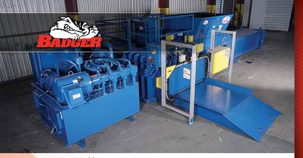
The Badger is the **WOrkhOrSe** in the narrow box line. It provides a superior MSW bale package as compared to any other baler manufacturer. It is a heavy duty baler that offers the highest baling forces in its class. The Badger offers feed hopper openings of either 65" (1651mm) by 74" (1879mm) or 65" (1651mm) by 94" (2387.6mm). MSW production rates up to 38 tons (34.4 tonnes) per hour.
