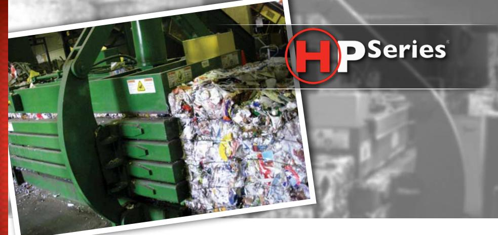
The HP 8240 MSW open end horizontal auto tie baler is designed with state of the art hydraulics that provides higher throughputs and densities, easy to use controls with multiple programs for full automation, enhanced safety features, a **SUPERIOF** structure for durability and simplified maintenance. The 4000lb (1815 kg) range bale weight provides for 60-70+ ton (54.4 - 63.5 tonnes) per hour throughputs.
