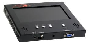
Bring the display to the source without having to move a 50" display. With the ability to not only test resolutions up to 1080p, 1920x1200 and 3D but the ability to learn any display's EDID. The AT-DIS7-PROHD is a testing device that can duplicate hot plug events and validate audio signal pressence. Ensure no time is wasted on an installation or tech call with the Atlona 7" Portable Testing Monitor.
