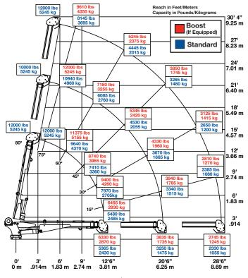
Weight of load handling devices are part of the load lifted and must be deducted from the capacity. Maximum 1 - part line capacity is 6000 lbs. (2720 kg). For greater loads, use 2 - part line.
