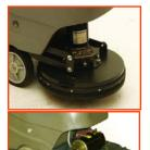
Low brush deck is ideal for cleaning around and underneath obstacles such as warehouse racks.
