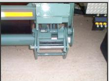
The Kann Commercial Side Loader can be easily converted to pick up most popular containers via a simple pin and rotating collar system designed into the carriage adaptor.
