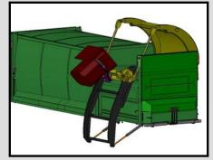
The Kann Commercial Side Loader with cart grabber mechanism option allows for collection of up to 96 gallon carts with optimal loading cycle time.
