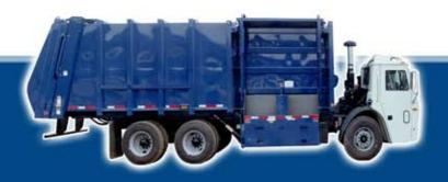
The Dual Swing-Link packing mechanism packs recyclables or any two commodities into two separate compartments and dual bubble tailgates allow the two body compartments to be emptied independently, for ease of unloading at the recycling facility.
