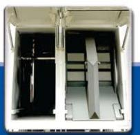
The Formula 4060 features a 40/60 split body with independent hydraulic systems for each compartment while maintaining an overall lower profile for better center of gravity and clearance from obstructions.
