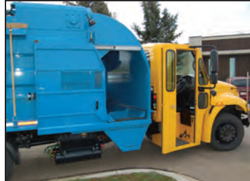
Dual steering stand up cab to collect with the traffic flow.
