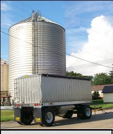
The Kann Pup Trailer has a steerable front axle to decrease tire wear and body stress under heavy loads. The steerable axle can be locked when backing.
