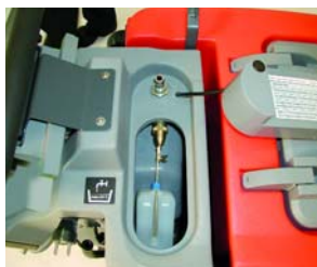
Large tank opening allows for fast fill and automatic filling systems.
