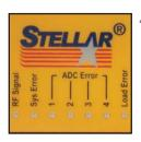
The new Stellar® CDT™ equipped cranes feature an enhanced safety system. If a device intended to monitor the capacity of the crane operates incorrectly, the crane will put itself into safe mode. Safe mode will allow the operator to work with the crane at a reduced speed until the safety device is in proper working order.
