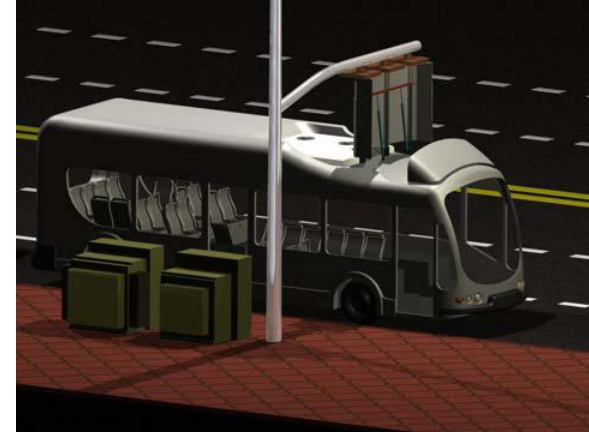
Charge mechanism deployed for charging
