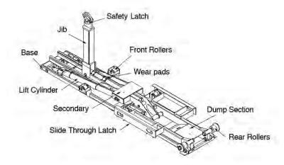
Base Section The base section of a Stellar Slider may also be called a sub-frame. All Stellar Slider Hooklifts are tied
