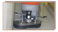
**Offset Brush Head:** The offset brush head allows for greater viewing of the area to be cleaned and allows for easier access along walls and underneath low profile objects.
