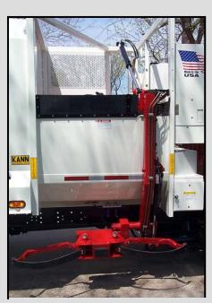
The Kann Automated Arm is stored within the legal width requirements and at cart height so the operator can achieve optimum loading cycle.
