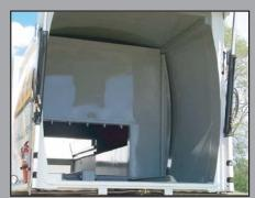
The full eject push out panel quickly travels the full length of the body and is engineered to eject all types of refuse and recyclables easily and completely clean.
