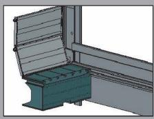
A) The hinged follower cover allows for constant loading without commodity falling behind the compactor blade.
