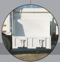
Low 35 inch Loading Height and Up To 2 Cart Tippers Per Trough
