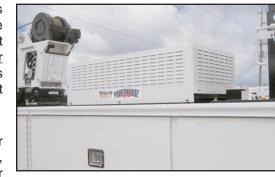
Conversely, the unit can be operated with the engine running. When the crane function selector is released, the truck charging system immediately begins the recharge cycle in the Powerhouse 24. Either way, with the chassis engine on or off, an intermittent (50%) duty cycle will allow a minimum of sixty minutes of use.
