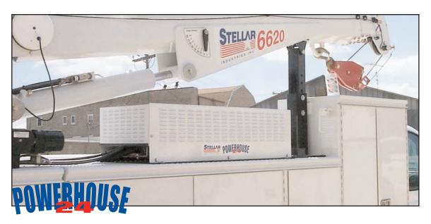
Market research and consumer demands has prompted Stellar Industries to develop the Powerhouse 24 hydraulic power supply. This unit allows the operator to manipulate the crane or other hydraulic equipment\* with or without the chassis engine running or when a pump and PTO is not applicable.
