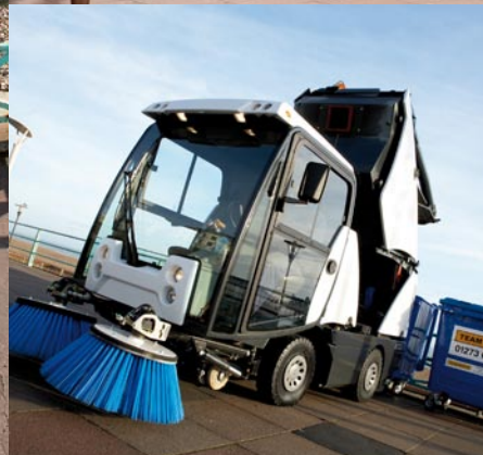
FAR LEFT Joystick control brushes extend an extra 3 ft for hard-to-reach area.
