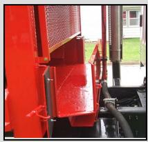
The Kann High Compaction Rear Loader has large cleanouts conveniently located on each side in the front of the packer body for easy access and serviceability.
