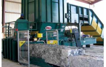
The Harris **Gorilla** is the **ECONOMICA** wide box two ram baler designed for medium volume applications for multiple materials. The **Gorilla** incorporates many robust features from the larger Harris two ram family including the automatic wire tie.
