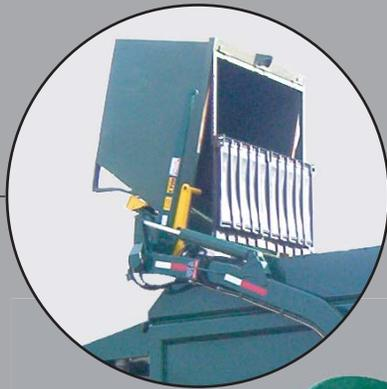
*The KA™ Allows For Collection Of Both Front and Rear Load Containers With The Same Front Loader*
