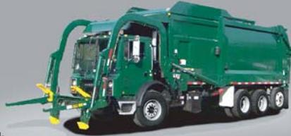
The **KANN Adapter** was designed to allow existing front load trucks to collect both standard front load and rear load containers up to 6 YD<sup>3</sup> capacity that meet ANSI Z245.6 standards.
