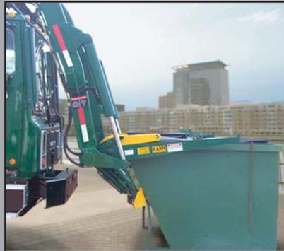
*The KA™ allows front loaders to also access rear load containers.*
