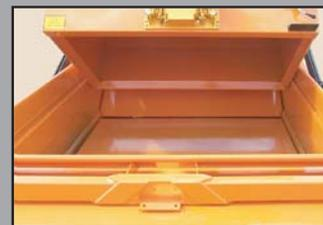
*Loading onto the follower cover allows constant loading while reducing cycle time.*
