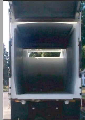
*The contoured blade smoothly follows the continuous uniform side walls from compactor to body, to prevent commodity falling behind the blade.*
