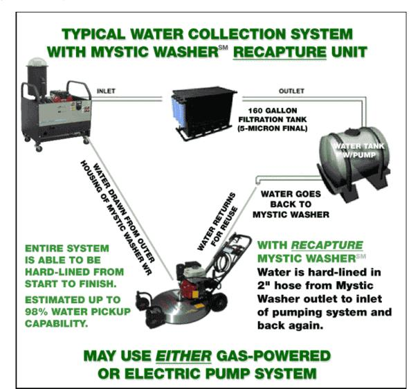
It is possible to reclaim a significant portion of used water with a standard Mystic Washer® unit. However, because it is not a hard-lined, totally contained system, it is impossible to collect and reuse the same amount of water as what is available with a Mystic WR machine.
