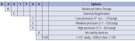
Example: RBE1720 with 1-1/2" body is a 1700 series regulator with balanced valve, an External Control line, and 1-1/2" NPT Valve body connection
