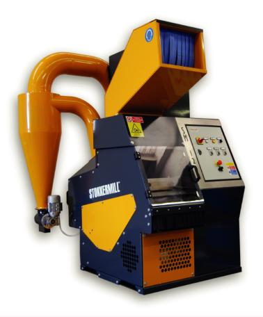
A compact low cost granulator perfect for most small to medium sized electrical cable granulating jobs. Robust and reliable with long service intervals due to the use of the self cleaning cyclone filter. Low power consumption of only 8.5 KW per hour.
